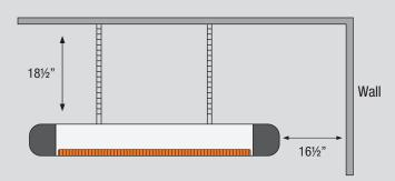
Locate stud in ceiling or wall and securely fasten bracket. Attach heater to bracket, adjust to desired position and tighten down. Must have minimum 71" clearance from the floor.
