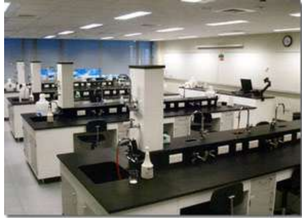
Chemistry lab floor is sealed to contain any spillage.
